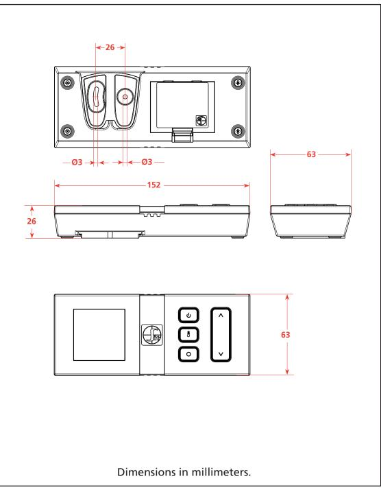
Fig. 24: PROFLAME transmitter dimensional drawing
