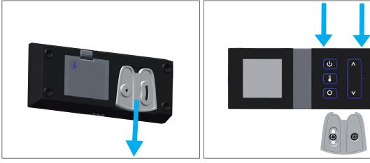
Fig. A: Detach the adapter from the body
