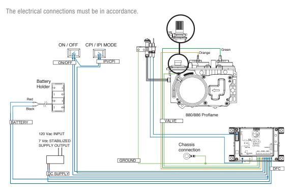
Proflame Standalone & 880/886 PROFLAME wiring diagram
