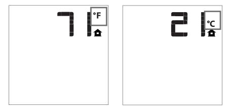
Fig. 6: Remote Control display in Farenheit and Celsius.
