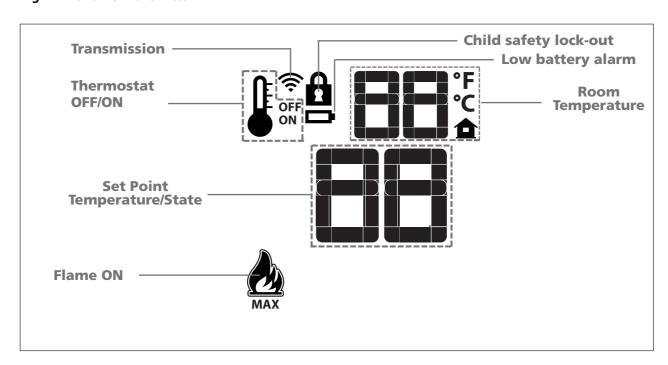
Fig. 2: Transmitter LCD display.
